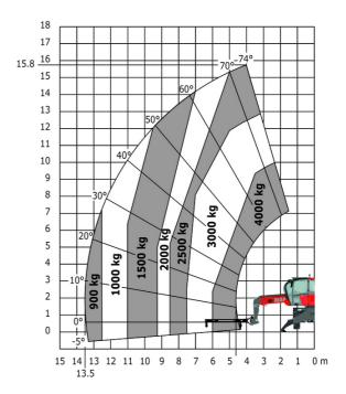
Machine on lowered stabilisers with 1500 kg jib with winch Machine on lowered stabilisers with hook 5000 kg (Metric) (Metric)
