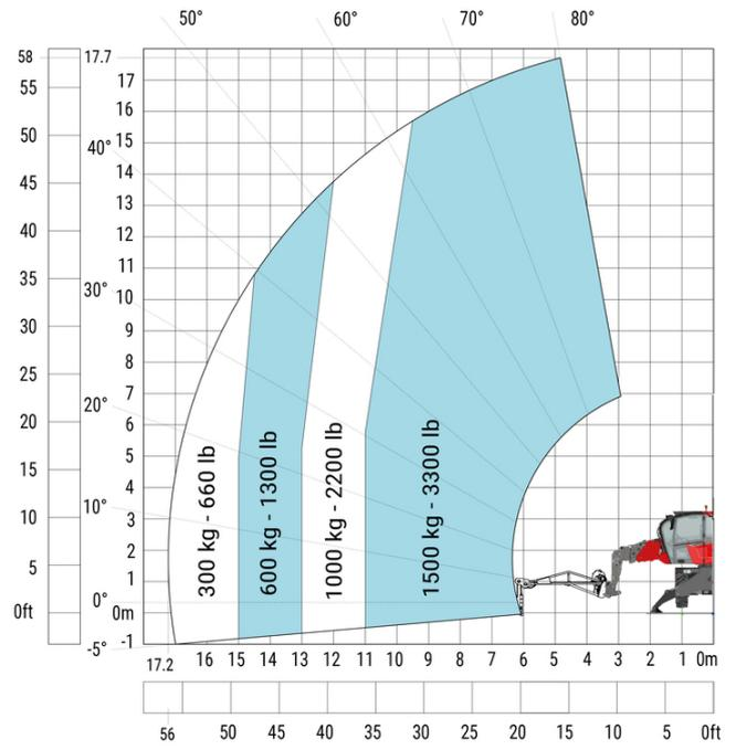
Machine on lowered stabilisers with 4000 kg jib (Metric)
