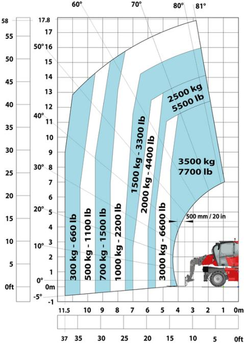
Machine on lowered stabilisers with forks Metric
