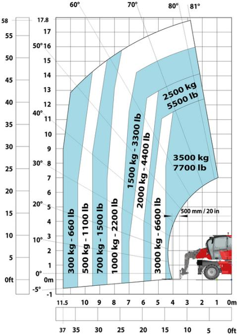
Machine on lowered stabilisers with forks Metric
