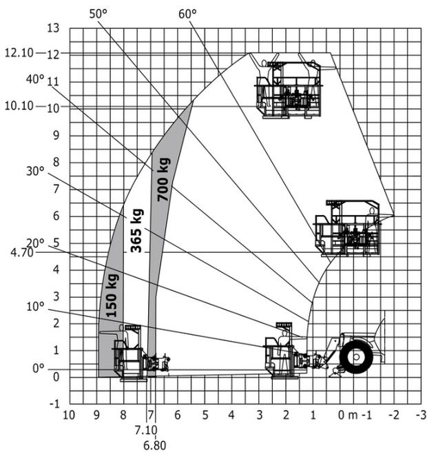
Machine on lowered stabilisers with underground mining platform (Metric)
