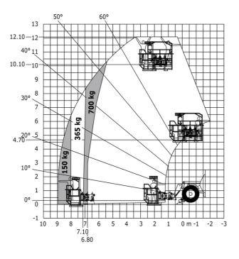
Machine on lowered stabilisers with underground mining platform (Metric)
