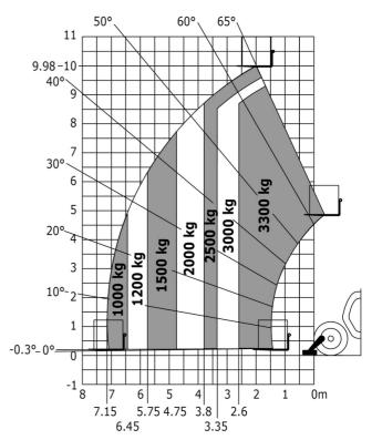
Machine on lowered stabilisers with tunneling platform (Metric)
