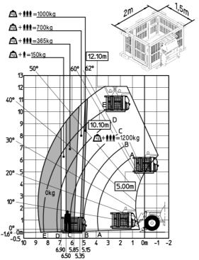
Machine on tyres with tyre handler TH 33 (Metric)
