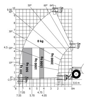
Machine on lowered stabilisers with tyre handler TH 33 (Metric)
